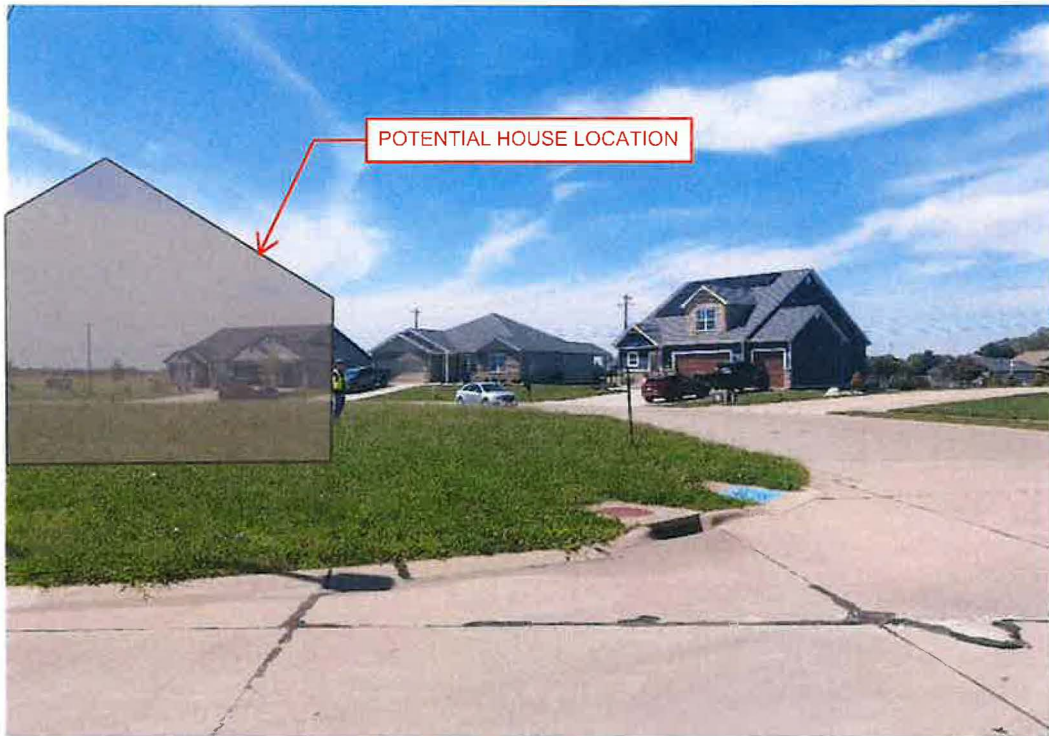
Photo 1: Sight-triangle looking north along Eisenhower with Field Technician representing building line.
